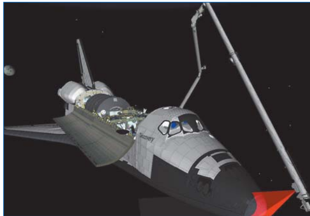
Figure 1. In this artist's rendering, Neptec's LCS scans the nose cone of the shuttle Discovery for potential damage to the shuttle's heatshield tiles.
